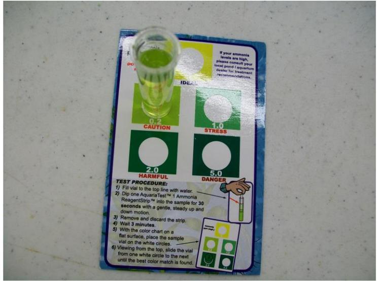
**High School Operation Water Drop kits** make it possible for students to test their local drinking water, control water samples and three other water samples for 13 different components (alkalinity, ammonia, arsenic, colour, heterotrophic plate count, iron, manganese, nitrate, residual chlorine, copper, pH, sulphate and total hardness). Students compare their results to the guidelines for Canadian Drinking Water Quality.
